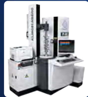
Bumeks gears are controlled by Klingenberg P40
