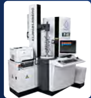
Bumeks gears are controlled by Klingenberg P40
